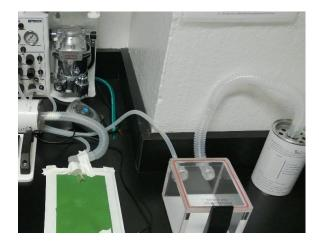
Before using the veporiser, weight the charcoals canister and record its weight, to determine if the canister needs to be replaced (follow the manufacturer instructions).
