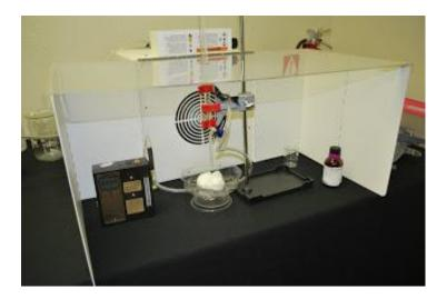
e.g. Laminar Flow Hood (Negative Pressure hood) with activated carbon filtered exhaust chamber.
